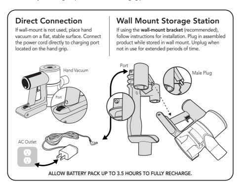
**NOTE:** During first use, run the battery all the way down to properly condition it, then charge fully. It takes approximately 3.5 hours to charge battery completely.
