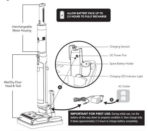
**SPARE BATTERY HOLDER charging:** insert the battery pack into the battery pack charging slot of the spare battery holder, connect the power adapter, the RED light will be on and start charging, the GREEN light will be on when it is fully charged.
